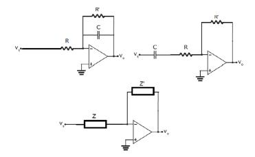
**Figure 5.11.** upper-left panel: inverting low-pass filter. upper-right panel: general inverting filter. lower panel: inverting high-pass filter.
