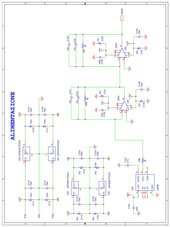
**Figure 5.6.** Scheme of the circuit prototype: page 3
