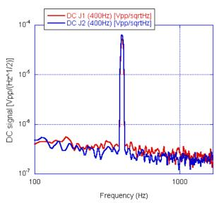
**Figure 5.25.** Response of the DC readout blocks (DC J1 and DC J2) at various offset and pulsating signals emitted by IR LEDs in the frequency band 100 Hz - 2 kHz.
