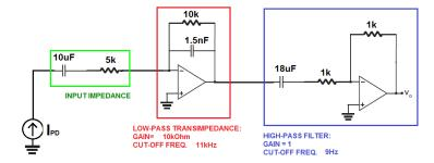
Figure 5.14. AUDIO readout blocks: first and second stage.
