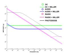
**Figure 5.12.** Plot of the magnitude of the input impedances of the DC, AUDIO and RADIO blocks, both considering ideal operational amplifiers or taking into account the Miller effect. Also the impedance which a photodiode sees toward the other photodiode is plotted.
