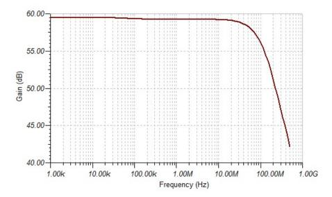
Figure 5.17. RADIO: transimpedance amplifier transfer function.
