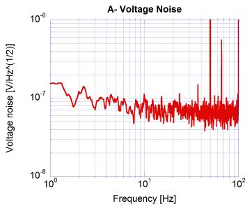
Figure 5.22. Voltage noise measured at the output of the AUDIO difference circuit in the frequency band 1 Hz - 100 Hz.
