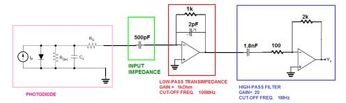
Figure 5.16. RADIO readout blocks: first and second stage.
