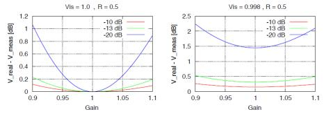
Figure 5.2. Electronic gain dependence of the squeezing detection efficiency. Taking the reflectivity to be R=0.5, depending on the initial squeezing value (10dB, 13dB and 20dB) and varying the electronic gain, the measured squeezing ( $V_{meas}$ ) diminishes with respect to the real one ( $V_{real}$ ). The situation is even worse if we allow a non perfect fringe visibility (shown in the right panel).
