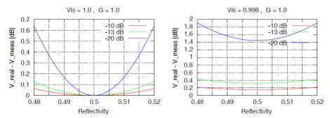
Figure 5.1. Beam splitter unbalance dependence of the squeezing detection efficiency. Taking the electronic gain to be G=1, depending on the initial squeezing value (10dB, 13dB and 20dB) and varying the beam splitter reflectivity R, the measured squeezing  $(V_{meas})$  diminishes with respect to the real one  $(V_{real})$ . The situation is even worst if we allow a non perfect fringe visibility (shown in the right panel).
