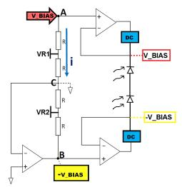
**Figure 5.8.** Bias circuit of the two phodiodes.  $-V_{BIAS}$  is obtained from the  $V_{BIAS}$  reference (5 V). Note the two points, VR1 and VR2, which are respectively at voltage  $V_{BIAS}$  and  $-V_{BIAS}$ : they are important in the DC-readout circuit.
