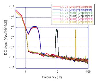
**Figure 5.24.** Response of the DC readout blocks (DC J1 and DC J2) at various offset and pulsating signals emitted by IR LEDs in the frequency band  $1 \ Hz - 100 \ Hz$ .
