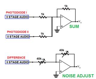
**Figure 5.15.** AUDIO readout blocks. *Top:* sum stage of the single-photodiodes readout blocks. *Bottom:* third stage of the difference photocurrent readout block.
