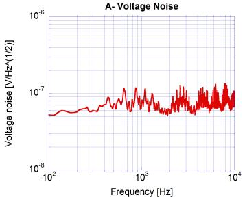
Figure 5.23. Voltage noise measured at the output of the AUDIO difference circuit in the frequency band  $100 \ Hz - 10 \ kHz$ .
