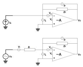
Figure 5.18. Schemes used for the noise calculations: on the top the transimpedance amplifier, on the bottom the voltage one.
