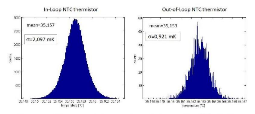
Figure 1.7. Measurement of the temperature stability obtained by a PID control loop.
