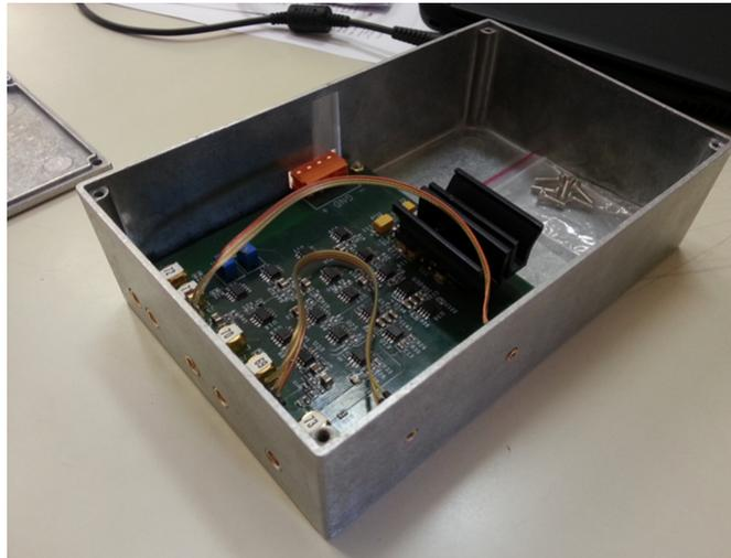
**Figure 5.21.** The first prototype of the homodyne detector electronic board. Two *ETX500T* photodiodes are fixed to the two small holes at the right side of the box, while on the other side there are standard *lemo* connectors for the various read-out blocks (DC 1 and 2, AUDIO sum and difference, RADIO difference, see sec. 5.1.3).
