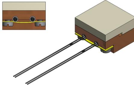
Figure 1.5. NTC thermistors dry assembly
