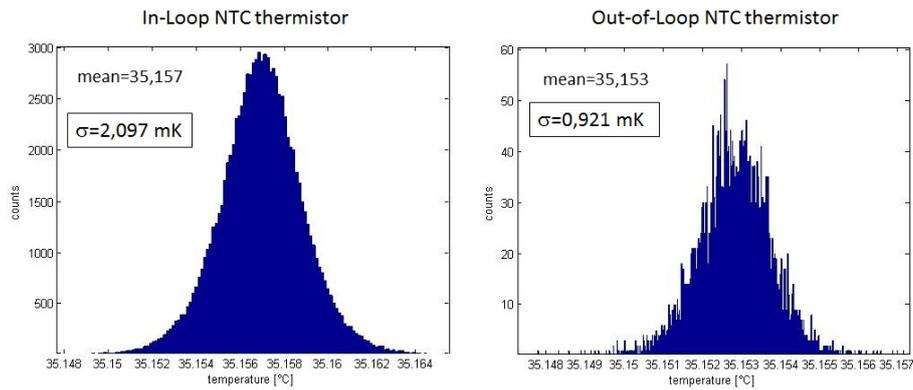
**Figure 1.3.** Temperature stability obtained by a PID control loop. The measurement was performed for a period of roughly 60 hours.
