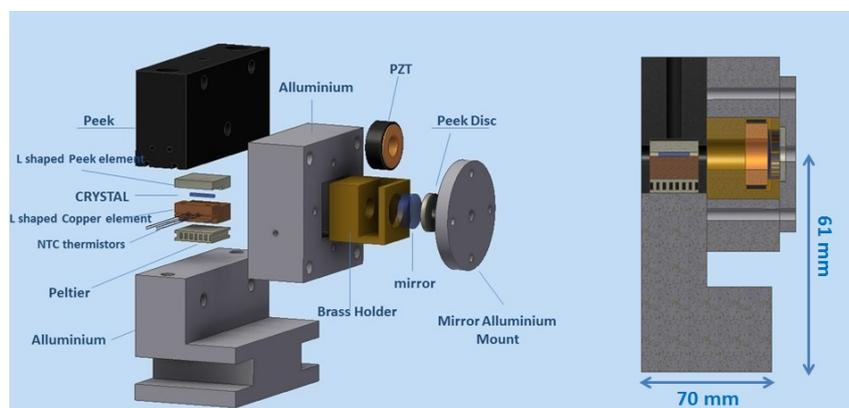
**Figure 1.4.** Left part: exploded CAD drawing of the prototype cavity. Right part: cavity dimensions.
