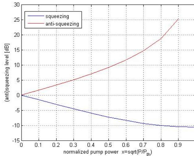
**Figure 1.2.** Taking into account the estimated value of losses, for  $x = 0.8$ , 10 dB is the maximum achievable level of squeezing.
