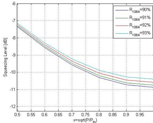
**Figure 1.1.** Levels of squeezing for several values of the outcoupler mirror IR power reflectivity. Value in table ?? are for  $x=0.8$ .
