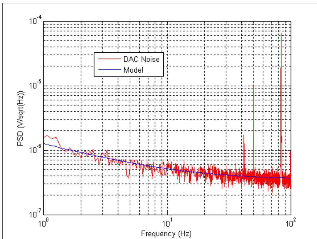
Figure 1 DAC noise ( $V_{out} = 0$  Vdc)
