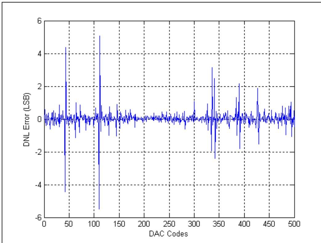
**Figure 2 DNL Error for a few DAC codes**
