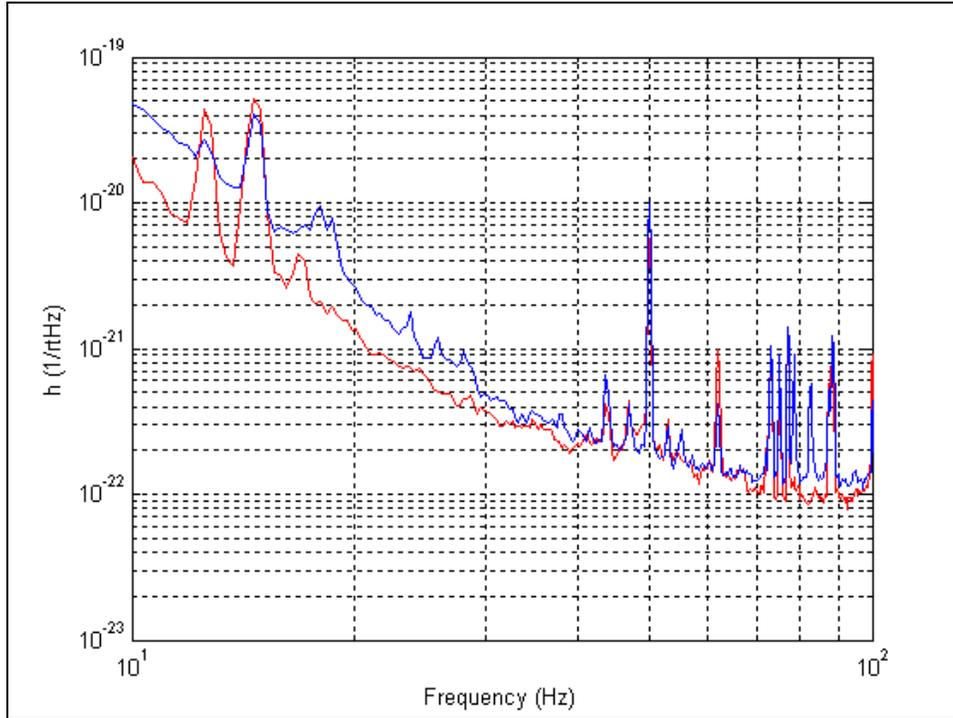
**Figure 8 Virgo Sensitivity with (red) and without (blue) shaping filters**
