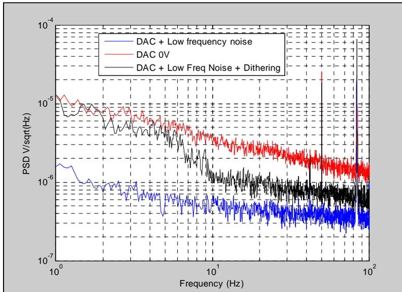
**Figure 6 Dithering Effect: up conversion is significantly reduced**
