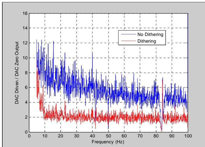
**Figure 7 Noise increase in respect with a DAC with zero input**
