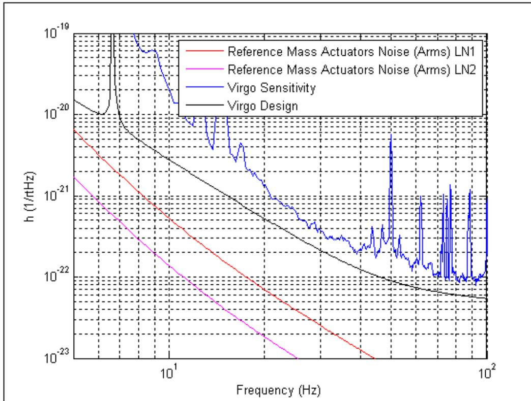
**Figure 14 Arms Reference Mass Actuators (LN1 and LN2)**
