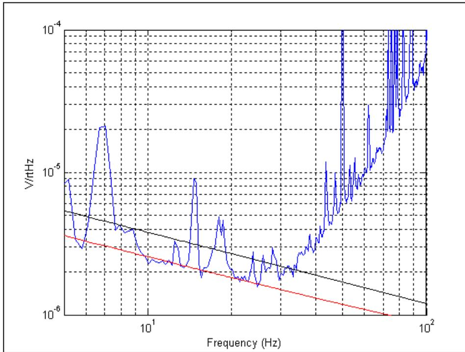
**Figure 9. DAC noise (blue) computed starting from measured sensitivity compared with original noise model (black) and with noise model reduced by 30% (red)**
