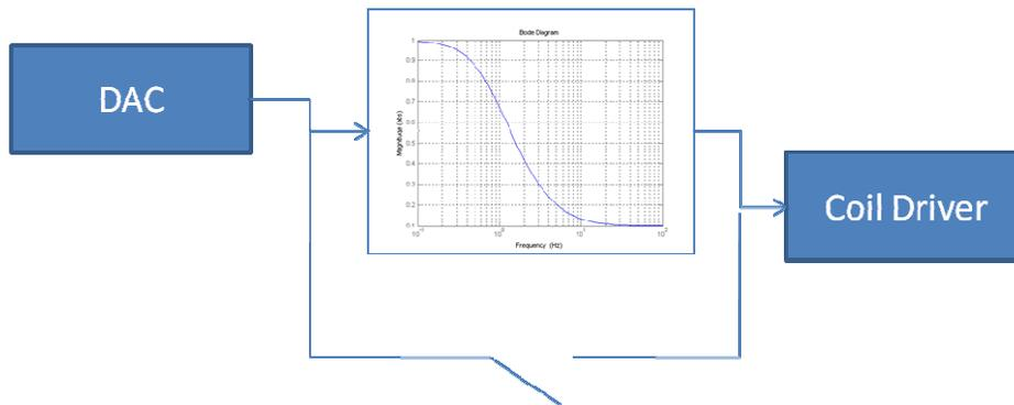
When lowpass filter is excluded (and also its highpass digital counterpart implemented in DSP), DAC noise contribution is increased by a factor 10.
