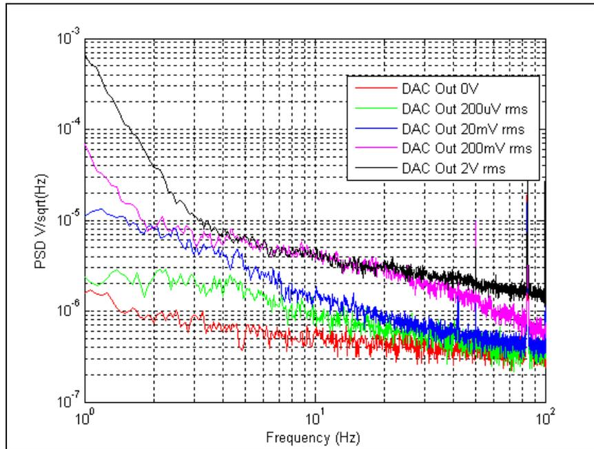
**Figure 3 Up conversion for different low frequency signal levels**
