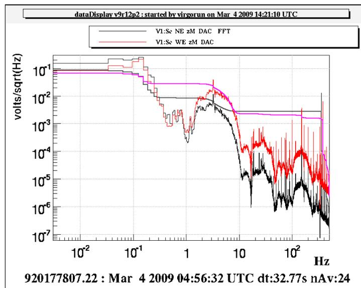
Figure 11 Comparison between DAC signal at WE (shaping filter on, dithering off, red line) and at NE (shaping filter off, dithering on, black line). Both rms values are below 100 mV.
