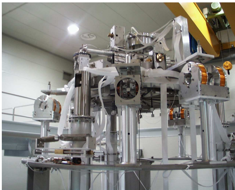
Figure 1 Superattenuator Top Stage
