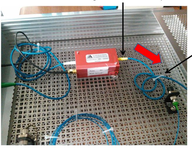
Too small radius of pig tail made a tension
