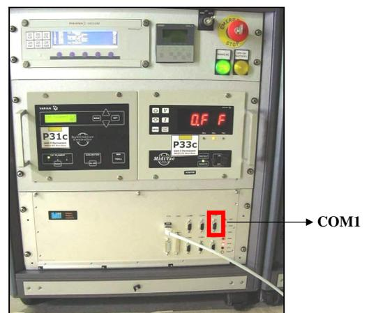
Fig. 2 : COM1 connector at OS9 crate front panel
