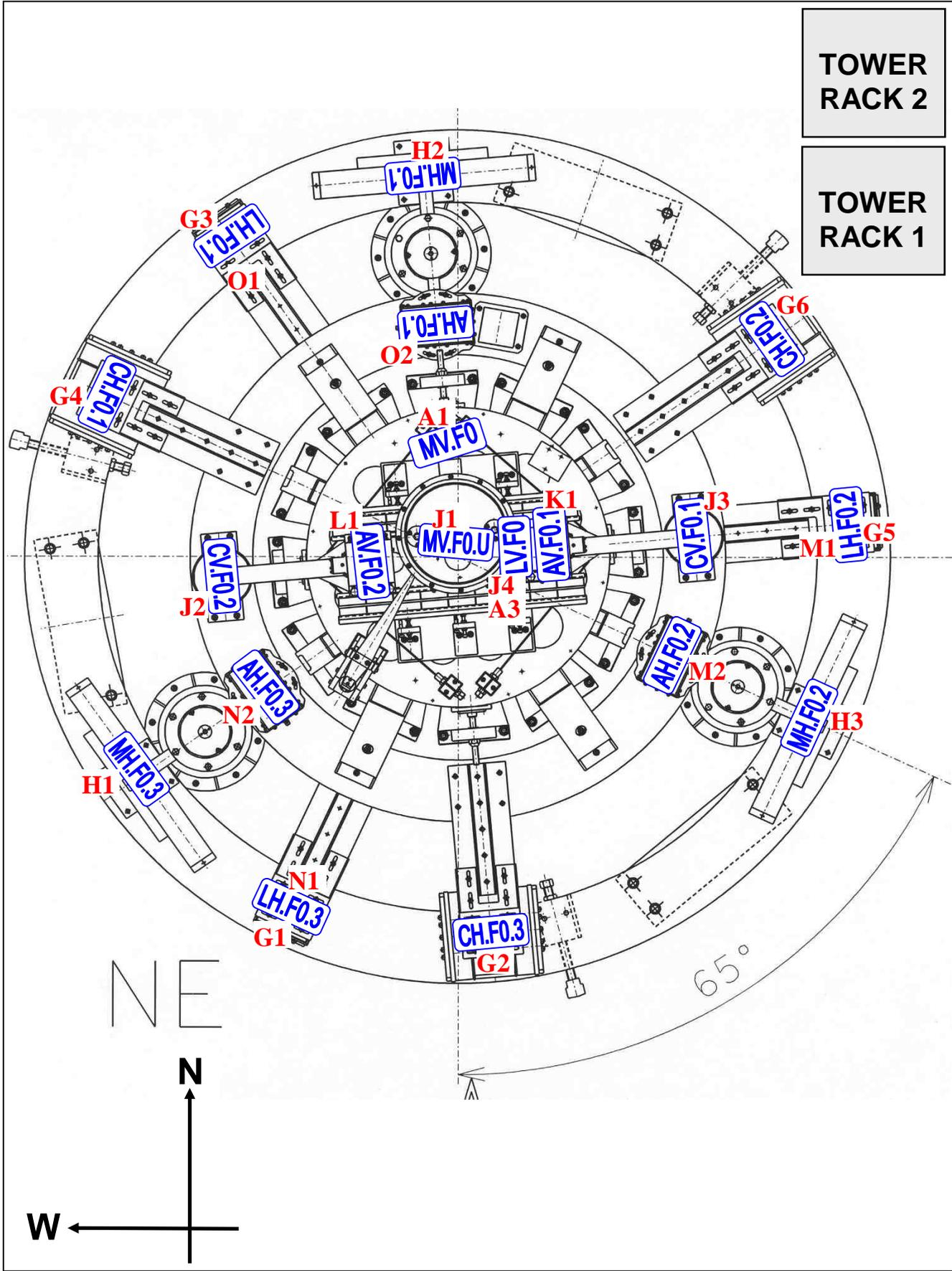
Cable arrangement along inverted pendulum (IP) legs and safety structure (SF) legs
