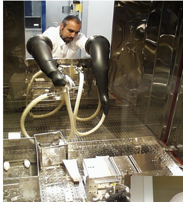
Cleaning with ultra-pure water inside the washing unit
