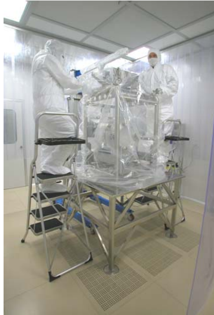
Packing of the payload in Clean Room with 2 plastic layers
