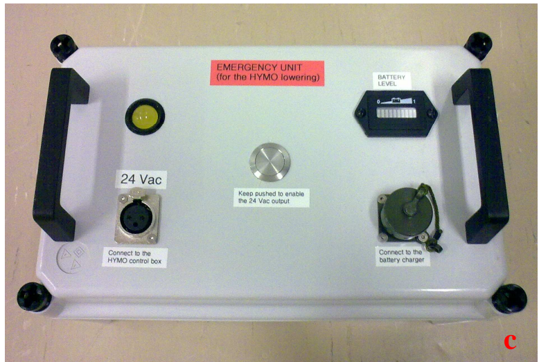
Fig. 6: Portable emergency unit: block diagram (a), inside view (b), external view (c).
