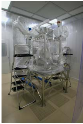
Packing of the payload in Clean Room with 3 plastic layers
