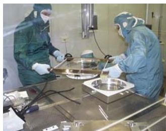
Preparation of mirror under a hood with laminar flow ISO 3 (class 1 US FD 209D)
