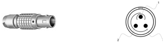
Fig 2: plug's picture and technical drawing (rear view) showing markings and pin numbers
