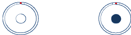
Fig.28: LEMO's single pin connector. Back (soldering side) view. Pin number assignment for receptacle (ERX.00.250.NTL, left) and plug (FFA.00.250.CLAC29, right)
