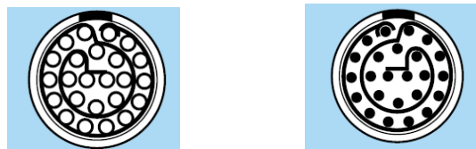
Fig. 19: receptacle and plug drawings of the selected 32-pin connector. Back (crimping side) view. Markings that allow to identify pins are clearly visible. Pin number assignment will be detailed later on.
