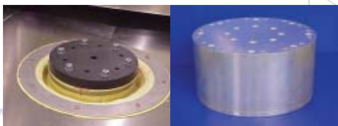
Seal test cabinet
