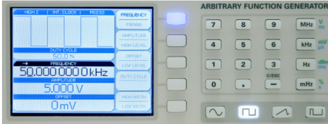
Fig. 4.3: Front view including display of the settings
