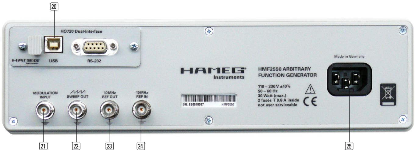
Fig. 2.2: Rear panel of the HMF2550 / HMF2525
