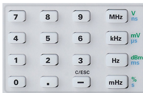
Fig. 4.2: numeric keypad and key's for unit's and escape
